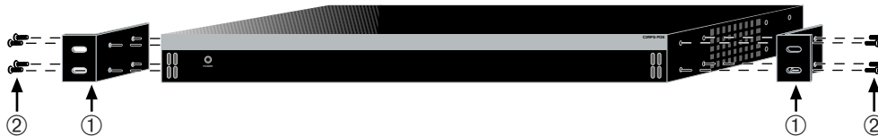
Figure 2-3 Attaching the Rackmount Brackets
